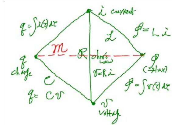
$$\begin{aligned}\phi &= q \\ \phi &= f(t) \\ \frac{d\phi}{dt} &= \dot{\phi} = \frac{d}{dt}f(t) \\ &= \left[ \frac{df(t)}{dq} \right] \frac{dq}{dt} = i \\ V &= \left[ \frac{df(t)}{dq} \right] i \quad \text{is memory resistor} \\ &\quad \boxed{\text{Memristor}}\end{aligned}$$
